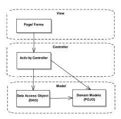
Figure 2: Model-View-Controller (MVC) technical architecture
