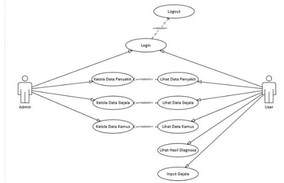
Gambar 1. Use-Case Diagram Sistem
