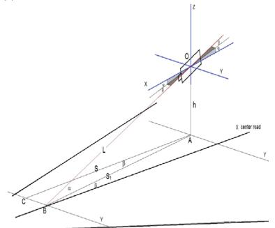
Picture (1) CCTV Geometry and Projection on Roadway
