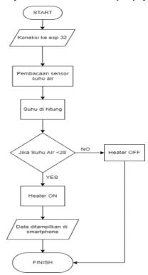
Fig. 15 Flowchart of How the System Works in the Temperature Monitoring Process Tilapia Fish Water.
