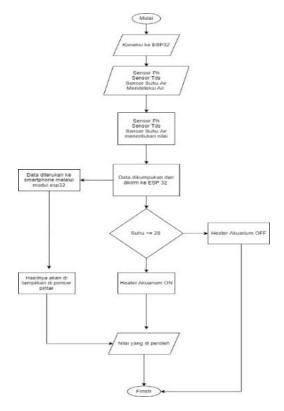
Fig. 14 Flowchart of How the System Works in the Process of Displaying Data to a Smartphone.
