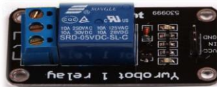
Fig 7. Relays (Source : https://www.Shopee.co.id )
