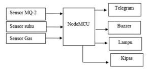
Fig 3. Block Diagram
