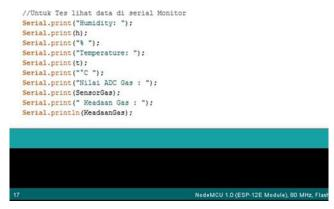
Fig 8 MQ-2 Code Sensor
