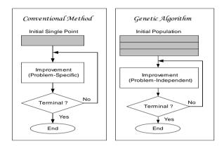
Figure 4. Comparison between Conventional Method and Genetic Algorithm<sup>[7]</sup>
